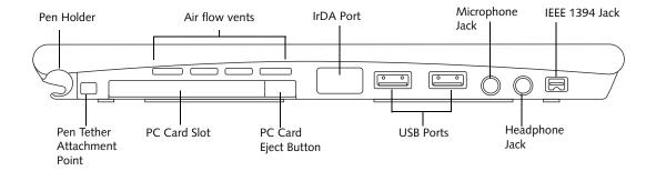
Figure 1-4 Stylistic ST4000P Series Pen Tablet PC Features (Top View)
